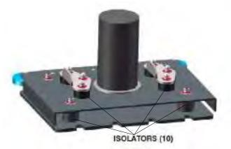
If any of the eight isolators show signs of wear, degradation or damage, contact your local distributor to replace all eight isolators.
