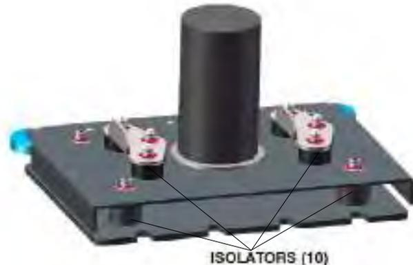
2. If any of the eight isolators show signs of wear, degradation or damage, contact your local distributor to replace all eight isolators.
